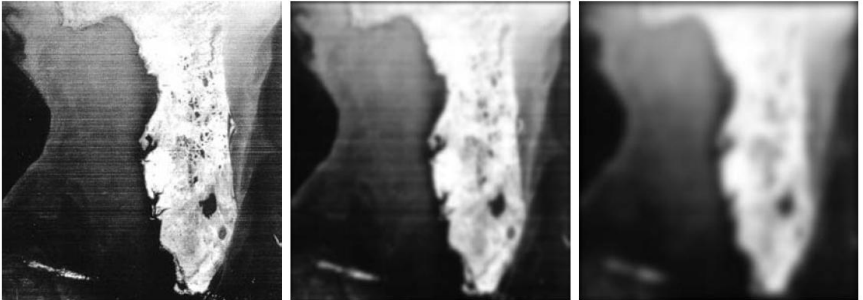
FIGURE 4.51 (a) Image showing prominent horizontal scan lines. (b) Result of filtering using a GLPF with D_0 = 50 . (c) Result of using a GLPF with D_0 = 20 . (Original image courtesy of NOAA.)
