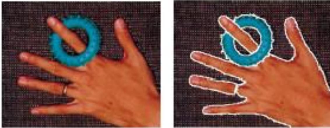
Figure 5.18 Mean-shift color image segmentation with parameters (h_s, h_r, M) = (16, 19, 40) (Comaniciu and Meer 2002) © 2002 IEEE.
