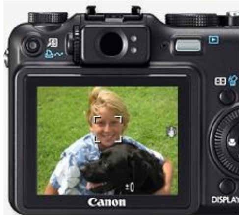
Setting camera focus via face detection
