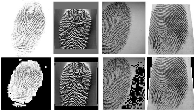
Fig. 1. 1st Row:Fingerprint Images from FVC2004 database, 2nd Row:Mean and Variance Based Segmented Images
