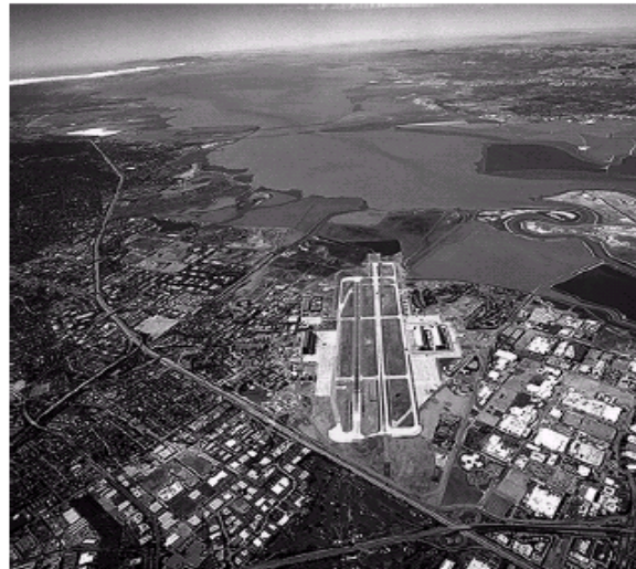
Result of Power law transformation c = 1, \gamma = 5.0 (high contrast, some regions are too dark)
