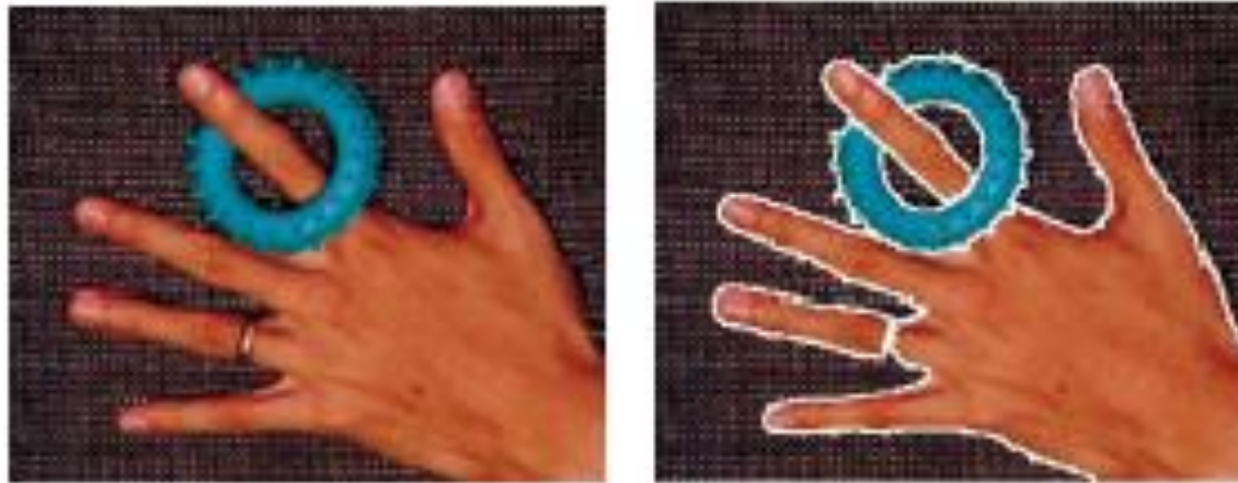
Figure 5.18 Mean-shift color image segmentation with parameters (h_x, h_r, M) = (16, 19, 40) (Comaniciu and Meer 2002) © 2002 IEEE.
